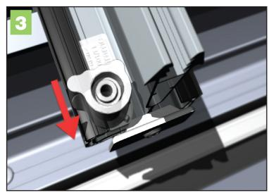
Slide the complete assembly down the glazing bar, using the fixing block as the 'stop'. Next, lift the polycarbonate panel into position and centralise it. If necessary pack it out on each side.
