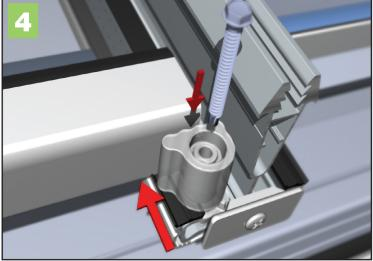
Ensure the glazing end profile sits snugly behind the grommet (if necessary slide the complete assembly up the bar to ensure contact. In exceptional circumstances the grommet may need trimming). Now, using the fixing provided screw down into the bar as shown.
