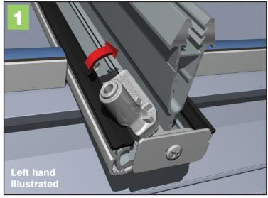
Snap off appropriate handed clip (left hand illustrated). Handing marked on base of clip. Line up the rounded edge on base plate next to central web of glazing bar then tuck neatly under gasket side of bar. Rotate clip into position.
