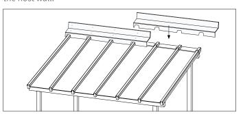
Align aluminium wall flashing with the panel corrugations, and position the upstand against the wall. Apply silicone to the back to act as a secondary water barrier, if desired.
