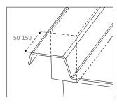
Position the first panel with the 'upper' edge corrugation resting on starter rafter, leaving a 50-150mm overhang. If the roof is free-standing, leave a 50-150mm overhang on the top edge also. Cut to length if necessary.
