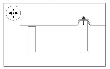
If the penultimate and end rafter is less than 600mm centre-to-centre, then the panel will need to be cut along it's length, and the end rafter installed 39mm lower than the other rafters, to allow the flat of the panel to sit level.
