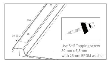
Drill 10mm holes along the outer corrugation. First and last holes should be located 30-50mm from the rafter's top and bottom edges.
