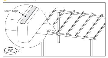
Apply the foam tape along the centre of each rafter to reduce friction and noise due to thermal expansion.
