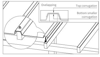
Drill 10mm holes through both panels, on the lateral overlap. As with first panel, the first and last holes should be between 30-50mm from ends, and intermediate holes no more than 500mm apart. Fix both panels together using the screws and washers specified. Start at the bottom and work your way up.
