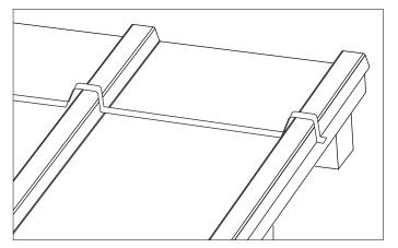
For improved weather-sealing of the wall flashing over the panels, a butyl tape can be applied to the top of the panels before the wall flashing is fitted.
