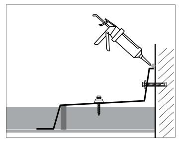
Wall flashings should overlap by 200mm, one corrugation.
